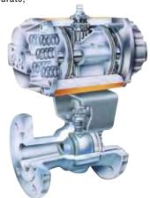
Piston tilting is prevented due to unique guide rods that always keep the pistons parallel with each other and perpendicular to the cylinder. This feature enables the Series 39 actuator to match the performance of diaphragm actuators in terms of high resolution. Internal friction is reduced with a nickel acetate-coated cylinder, low coefficient-of-friction acetal resin bearings and a special permanent lubricant with corrosion inhibitors.
