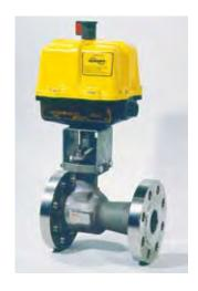
Series CPT 94 control valve shown on page 6 has been certified by third party testing, allowing less than 25 ppm leakage, whereas EPA requirements are 500 ppm. Selfadjusting stem seals with multiple Belleville washers make this valve ideal for throttling toxic chemicals.
