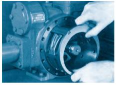
Easily replaceable liner restores efficiency.
