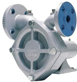
The frame mount design requires a baseplate, coupling, and coupling guard and utilizes a direct drive configuration so the pump runs at motor speed. With a frame mount design, the user has the flexibility to choose from a variety of motor sizes. FF- & DLF-models 075, and 150 produce higher differential pressures than F-Model pumps and are commonly used in Autogas applications.
