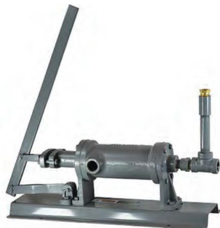
Piston type hand pump for filling portable and motor fuel cylinders. Connects to 1" inlet and 3/4" outlet. Weighs 55 lbs. and pumps 6 gallons per minute at 40 strokes per minute.
