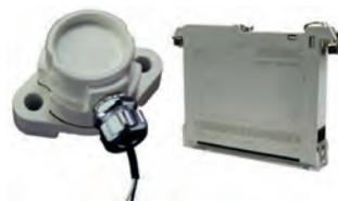
This transmitter is designed to fit Rochester model 6342 and 6360 Magnetel float gauges with 8" dials. The transmitter provides a current output of 4-20 mA proportional to the liquid volume in a horizontal storage tank. Safety barrier provides intrinsic safe outputs.
