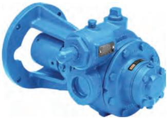
These motor-speed pumps offer higher capacities than the LGF1/B1 Series pumps. They are suited to a variety of small transfer jobs, but are especially popular for multi-station cylinder-filling systems. They are equipped with a built-in relief valve and are fitted for both LP Gas or anhydrous ammonia service. These pumps are designed for foot-mounting. All of the pumps are equipped with replaceable cylinder liners and end discs, permitting rebuilding of the pump to like new condition.
