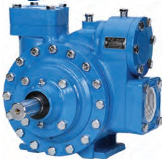
These workhorse pumps have long been popular for a broad range of service on bobtails, transports, vaporizers and bulk transfer service. The LGLD2 and LGLD3 are particularly suited to bobtails, because they offer a double shaft extension. This permits use of the pump by either right or left handed PTO rotation simply by reversing the position in which the pump is mounted.
