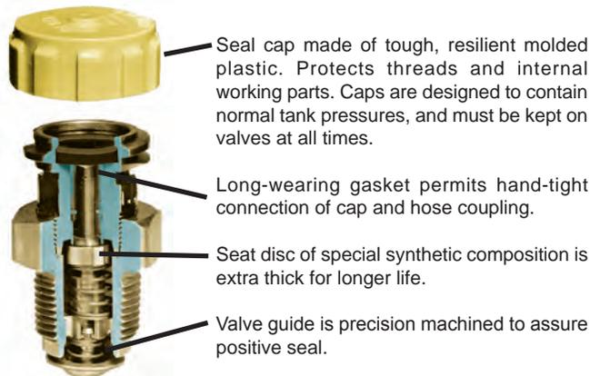
**WARNING:** Under normal conditions, the useful safe service life of a pressure relief valve is 10 years from the original date of manufacture. However, the safe useful life of the valve may be shortened and replacement required in less than 10 years depending on the environment in which the valve lives. Inspection and maintenance of pressure relief valves is very important. Failure to properly inspect and maintain pressure relief valves could result in personal injuries or property damage.
