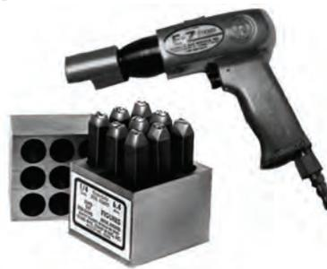
Stamps the date clearly as required by DOT regulations. Takes less than 30 seconds to stamp complete date on a cylinder. Dies are 3/8" square and print 1/4" characters. Requires only 60 psi air pressure for operation.
