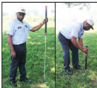
For boring test holes near buried gas lines or underground tank. 44" bar allows for sufficient depth in order to drop a gas detector probe into the ground for testing. Use with Sensit Technologies Track-IT III with sampling hose.
