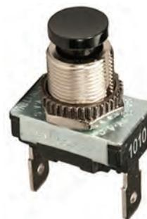
Heavy-duty, for either 6 or 12- volts. Has two binding head screw terminals. Mounting stem has 7/16-28 thread, is 3/8" long
