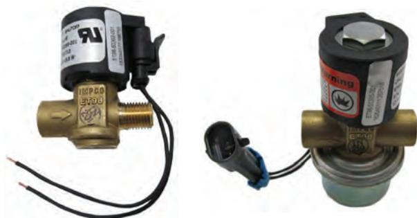
The Model ET98 is an electrically operated safety shutoff valve suitable for high pressure up to 315 PSI for LPG liquid, LPG Vapor or Natural Gas Vapor. It is normally closed Straight-Through Lockoff, opened with 12V DC.
