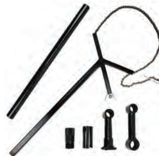
Special tools for removing or installing valves in DOT Cylinders.
