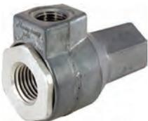
The universal design of this valve allows it to be used as a SUPER QUICK EXHAUST VALVE or a SHUTTLE VALVE. With the molded shuttle design, the Super Quick Exhaust valves have an operating range as low as 1 psi to 150 psi.
