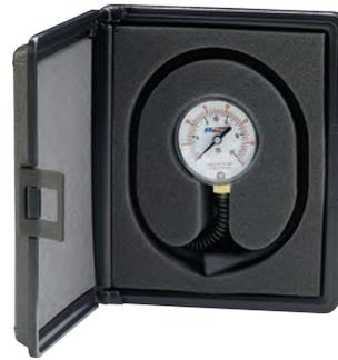
This kit provides the equipment necessary for checking regulator delivery pressure (low pressure) at the appliances. The basic set contains a 2424A-2 low pressure gauge and a 3 foot 3/16" O,D, flexible synthetic rubber tube. Adapters are also available.
