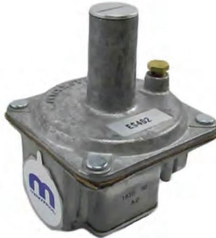
The IMPCO IMP Series of Regulators are low pressure, dry gas regulators intended for use with propane or natural gas. Typical applications include all types of stationary, gas-fired appliances and equipment utilizing a low-pressure gas supply. The IMP Series regulators feature a unique conical valve design, which permits low resistance straight-through flow. This design provides high flow at low pressures and enable the regulator to handle large capacity appliances with limited supply pressure.
