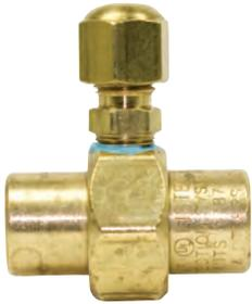
Low cost, permanently installed fitting between tank service valve and first stage regulator providing leak test capability without the use of tools. Eliminates the need to discard pigtail to access tank pressure. Easily installed with adapter such as male POL x 1/4" F.NPT and 1/4" female POL x 1/4" M.NPT.
