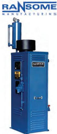
The RW Series vaporizer consists of a vertical ASME rated pressure vessel which is submerged in a water bath. The water is heated by a gas fired burner which consumes a small amount of vapor from the vessel to develop the heat required for vaporization.
