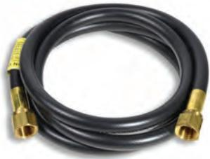
LP Gas Vapor Hose Assemblies are factory assembled in 3/8" hose I.D. and 1/4" hose I.D. in various lengths and end fitting configurations. These hose assemblies are rated for 350 PSI working pressure. Vapor service only.
