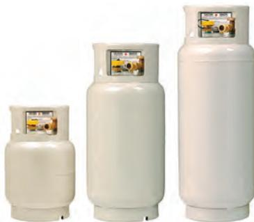
Standard cylinder fitted with liquid service valve, relief valve, float gauge, 20% outage valve. Filler valve and safety coupling installed.
