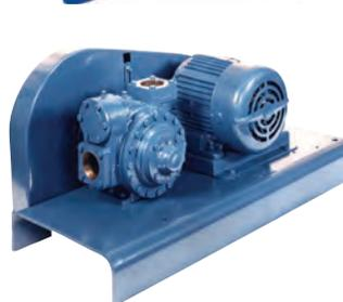
These units have high torque V-belts and quick disconnect sheaves. Sheaves are thinner, which puts them closer to the bearings, reducing the stress on both motor and pump shafts. Sheaves and hubs are a two-part assembly that comes apart easily. Units come complete with belt guard pump mounted to base plate, and a motor.
