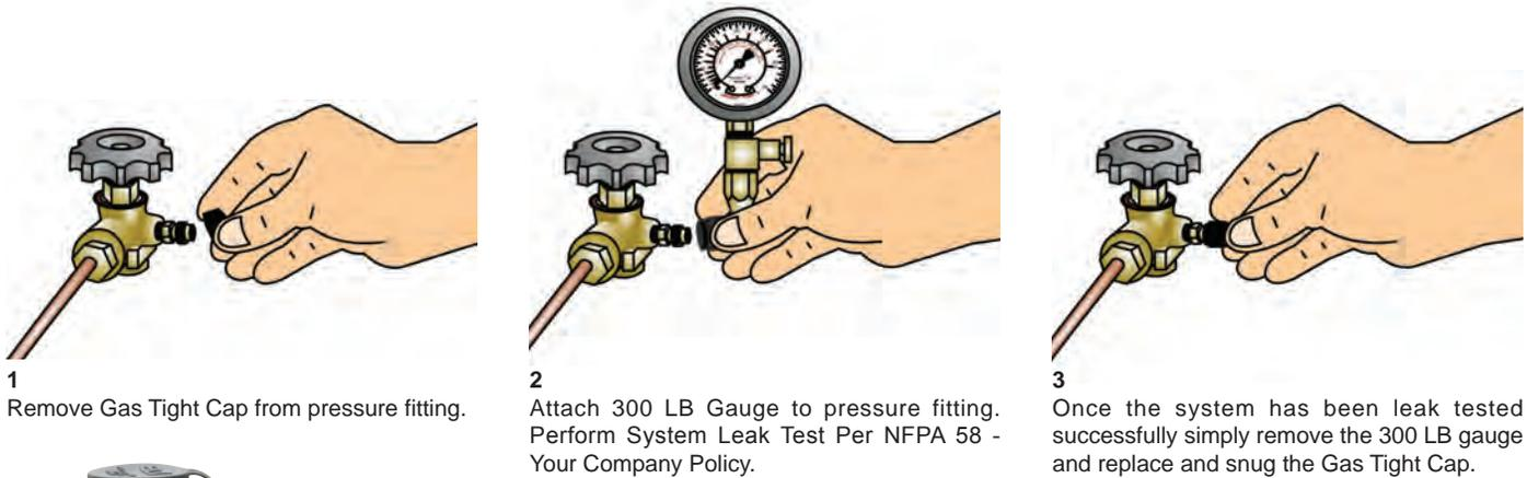
1 Remove Gas Tight Cap from pressure fitting.
