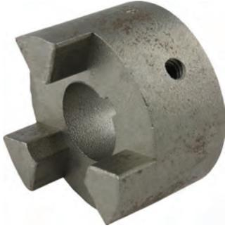
These couplings offer standard shaft-to-shaft connection for general industrial duty applications. Standard L-Type coupling hub materials are sintered iron. Sizes range from L035 to L276. These couplings require no lubrication and provide highly reliable service for light, medium, and heavy duty electrical motor and power transmission applications.
