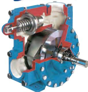
Blackmer's LGLD4 pump is fitted with a special cavitation suppression liner for optimum performance & extended service life. UL listed for handling butane, propane & anhydrous ammonia, this durable pump is ideal for rapid loading & unloading of transports and bob-tails or bulk plant service. Flow rates range from 130 to 270 GPM with differential pressures up to 125 psi.
